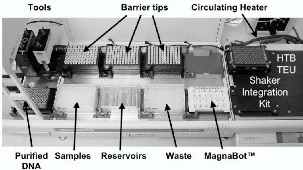
Deck layout for purifying DNA on the Biomek<sup>®</sup> 2000 workstation using DNA IQ<sup>™</sup> chemistry.
