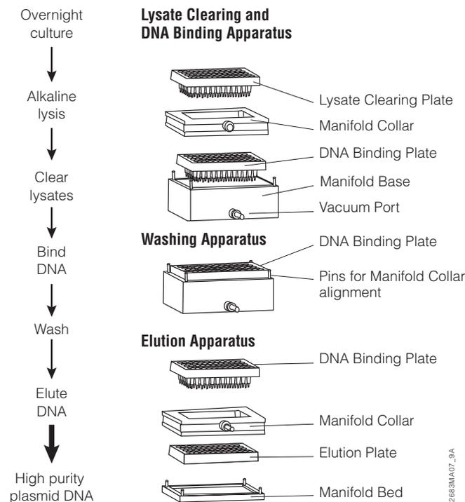
**Figure 1. Protocol overview.** Flow diagram of plasmid DNA isolation and purification using the Wizard® SV 96 Plasmid DNA Purification System. See Figure 2 for close-up view of the enhanced tip design of the Wizard® SV 96 Plate.
