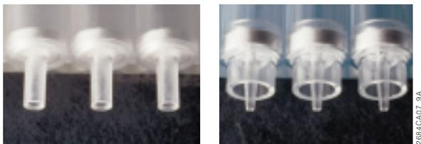
**Figure 2. Plate tip design comparison.** Photographs show increased tip aperture and absence of skirt for the Wizard® SV 96 Plate tips (left) versus the tips of a second commercially available 96 well plate (right).
