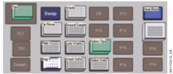
**Figure 3. Deck layout of the Biomek® FX workstation for the deep-well plate method using the Wizard® Magnetic 96 DNA Plant System protocol.**
