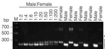
**Figure 5. Cross-contamination assay results.** Samples of blood from one female who never had a male child and one male subject were purified in alternating wells using the MagneSil® Blood Genomic, Max Yield System. The purified DNA was then amplified with *DYS214*-specific primers. Dilutions of male DNA into female DNA are shown, followed by alternating male and female DNA that was purified and amplified in adjacent wells. None of the female samples showed Y chromosome-specific products.
