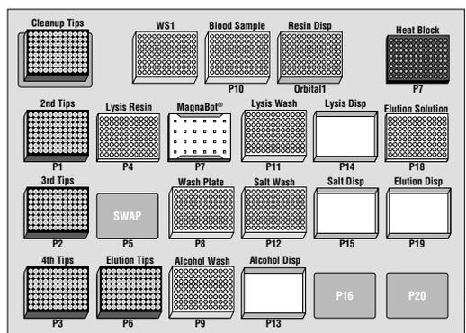
**Figure 1. Example deck layout of the Biomek® FX instrument.** Layout for the MagneSil® Blood Genomic, Max Yield System. Deck layouts may be different on different instruments and depend upon the individual instrument's configuration.
